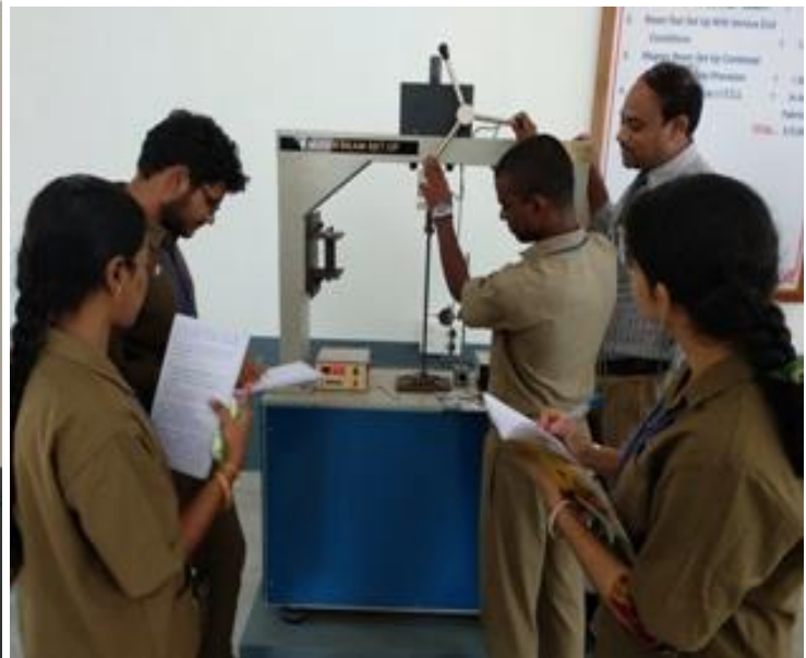
WAGNER BEAM SET UP COMBINED WITH COLUMN TEST PROVISION
